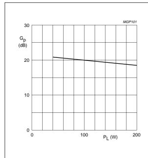
Class-B operation; V<sub>DS</sub> = 50 V; I<sub>DQ</sub> = 100 mA; R<sub>GS</sub> = 15.8  $\Omega$ ; f = 108 MHz.
