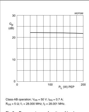
Fig.9 Power gain as a function of load power; typical values.
