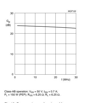
Fig.15 Power gain as a function of frequency; typical values.
