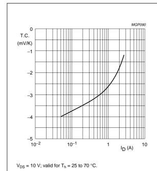
Fig.4 Temperature coefficient of gate-source voltage as a function of drain current; typical values.
