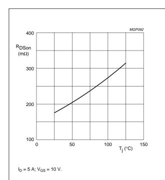
Fig.6 Drain-source on-state resistance as a function of junction temperature; typical values.
